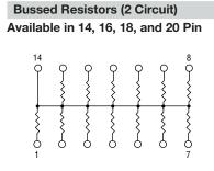
These models incorporate 13, 15, 17 or 19 thin-film resistors of equal value, each connected by a common pin.
